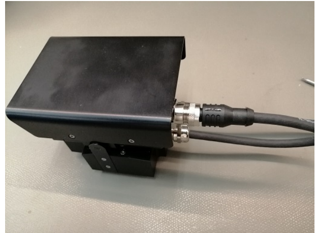
6 Connect the cable from the PTU to the camera, the retrofit is now complete
